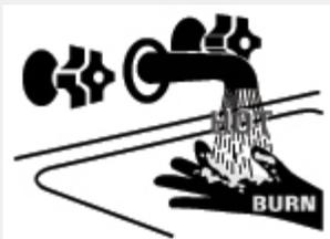
Because higher temperatures increase the risk of scalding, if you set the thermostat(s) higher than 120°F, Thermostatic Mixing Valves at each point of use are particularly important and recommended. Refer to the scald chart in your Owner's Manual.
